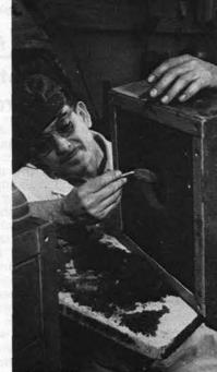
SMALLER PIECES for foundry casting are prepared in small "bench molds." Here Ramon Armijo smooths section of mold.
